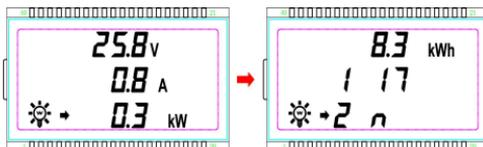
Display: Voltage/Current/Power/Consumed energy/Load working mode-Timer1/Load working mode-Timer2
